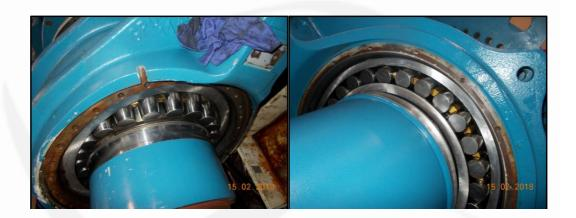
2. Cleaning the points of corrosion and protection of the areas without paint.
